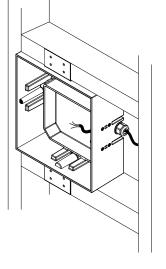
Install construction sleeve ("sleeve") inside the wall using provided L-brackets, mounting to structural supports (e.g., 2"x4" (50 mm x 100 mm) framing studs). For lighting in the downward direction, ensure the arrow in the sleeve is pointing upward.
