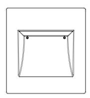
10. Use the included fasteners to attach the faceplate to the housing.
